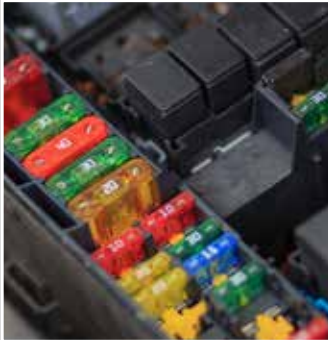
Inspection of car fuses – color and material
