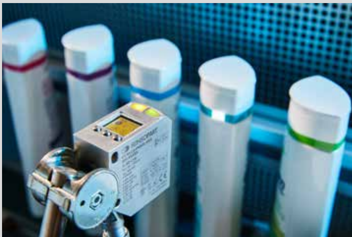
Color detection of packaging elements
